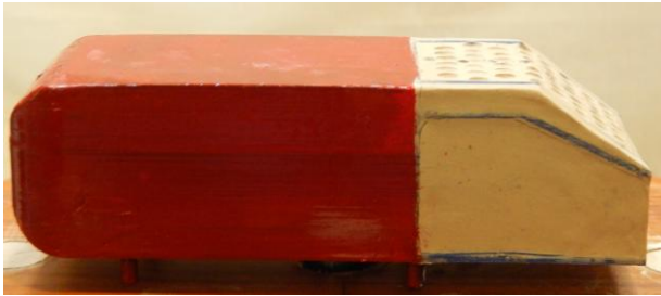
Figure 3. The image shows the 3D Printed Ahmed Body after surface finishing works were done, clay was applied and dimples were imparted.
