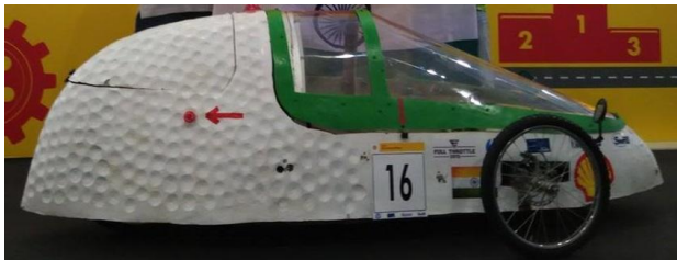
Figure 7. The dimpled super-mileage vehicle by ‘Team Go Viridis’ at ‘Shell Eco Marathon Asia 2015’
