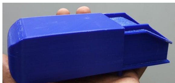
Figure 2. The 3D Printed Ahmed Body with reduced area of cross section at the rear. The image shows how the model looked before surface finishing works were done and clay was applied.
